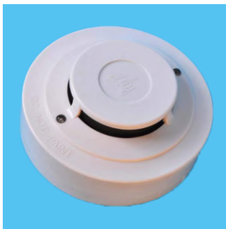
SMOKE DETECTOR Model DFS513 Operated volt-9VDC-35VDC; Sensor:Optical sensor; Sensitivity-0.15 dB/m( \pm 0.03 dB/m); Standby current: \leq 50\mu A (2 wires); Alarm current: \leq 50mA ;
