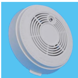
SMOKE DETECTOR Model DFS424 Operated voltage-9V Battery(include); Sensor:Optical sensor; Sensitivity-0.086DB/M to 0.140DB/M; Alarm sound: \geq 85dB(3M) ;
