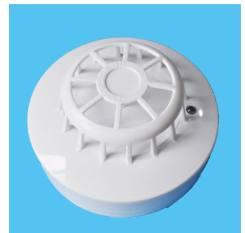
HEAT DETECTOR Model DFT518 Operated volt-9VDC-35VDC; Temp.Trip Point-57°C(135°F ); Standby current: \leq 50\mu A (2 wires); Alarm current: \leq 50mA ;
